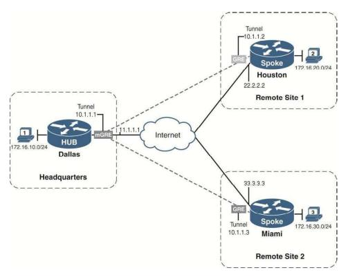
Multipoint GRE (mGRE) tunnels are similar in construction to point-to-point GRE tunnels with the exception of one command: the **tunnel destination** command. Instead of declaring a static destination, no destination is declared, and instead the **tunnel mode gre multipoint** command is issued, as shown in the example below (on the Dallas router):
