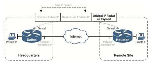
The Internet routers forward the new IP packet just as they would any other traffic, landing it at the Houston router. The Houston router removes the outer IP packet header to expose the original IP packet destined from Host A to Host B. The Houston router can then route the original packet out its LAN interface toward Host B.
