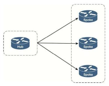
DMVPN clouds are, at their core, hub-and-spoke networks. The DMVPN hub router acts as the central aggregation point for all of the spoke routers that connect to it in its DMVPN cloud. In the NHRP network created in the first section, the Dallas router is considered the hub of the DMVPN cloud, and Houston and Miami routers are the spokes.
