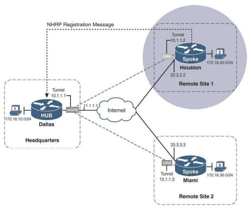
With the help of the **debug nhrp packet** and **debug nhrp detail** commands on both Dallas and Houston, the registration process can be observed in real time. Once Houston's tunnel interface comes online, Houston sends an NHRP registration packet to Dallas. It knows Dallas is the NHS because Dallas's IP address is identified in the **ip nhrp nhs 10.1.1.1** command on Houston's tunnel interface. This NHRP registration packet is shown in the debugging output below:
